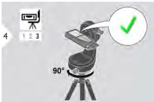
Rotate the device clockwise  $90^\circ$ . Follow the instructions on the display. Levelling is finished when OK icon appears on the display.
