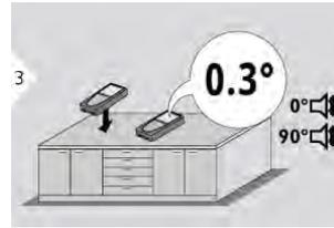
**i** Displays inclinations of 360°. Instrument beeps at 0° and 90°. Ideal for horizontal or vertical adjustments.
