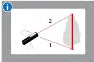
The height is calculated based on trigonometric functions with 1 known length and 1 measured angle.
