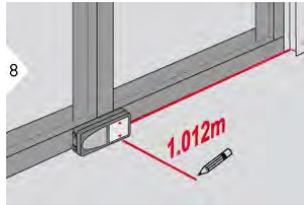
Move device slowly along the stake out line. The distance to the next stake out point is displayed.
