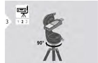
Rotate the device clockwise  $90^\circ$ . Follow the instructions on the display.
