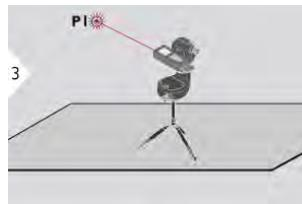
Define a point to be measured in a distance more than 8 m. Aim at defined point and press DIST button to start the 5 seconds countdown to measure.
