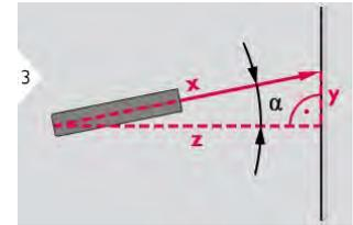
Aim laser at target (up to 360° and a transverse tilt of ±10°).
