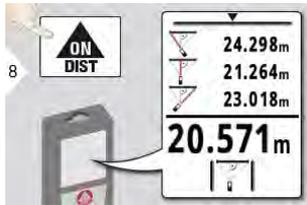
**i** The result is shown in the main line and the measured distance above. Pressing the measuring key for 2 sec in the function activates automatically Minimum or Maximum measurement. We recommend to use the pythagoras only for indirect horizontal measuring. For height measuring (vertical) it is more precise to use a function with inclination measurement. Use Down navigation key to take over values in the main line for sending via Bluetooth®
