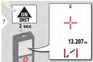
**i** If chosen permanent measurement for second target point, the actual tie distance is displayed.
