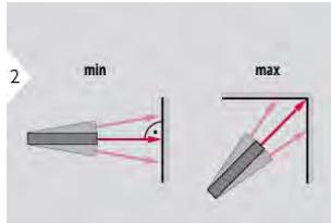
Used to measure room diagonals (maximum values) or horizontal distance (minimum values).
