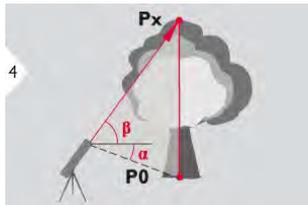
Aim laser at upper points and angle/height tracking starts automatically.
