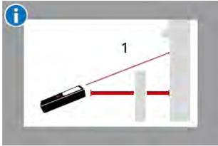
The horizontal distance is calculated based on the trigonometric function cosine with 1 known length and 1 known angle.
