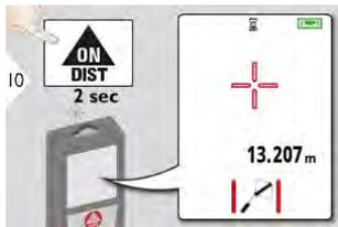
If chosen permanent measurement for second target point, the actual tie distance is displayed.
