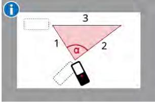
The angle is calculated based on the cosine rule with 3 known side lengths of a triangle.
