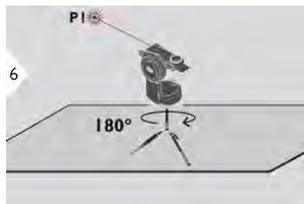
Turn the device by 180°. Aim again at defined point and press DIST button to start the 5 seconds countdown to measure.
