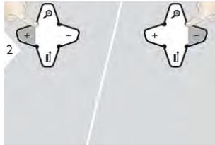
The next measurement is added to the previous one, respectively subtracted from the previous one.
