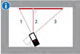
The distance is calculated based on the Pythagorean theorem with 3 known lengths of 2 right-angled triangles.
