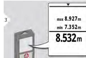
The minimum and maximum distance measured is displayed (min, max.). The last value measured is displayed in the main line.
