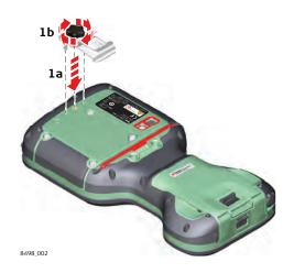
Fixing the utility hook (GHT68) step-by-step
