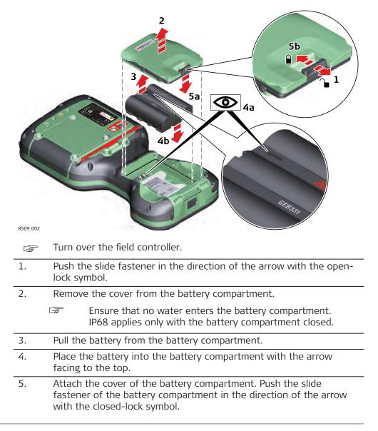
Insert and remove the battery on the GS07 step-by-step
