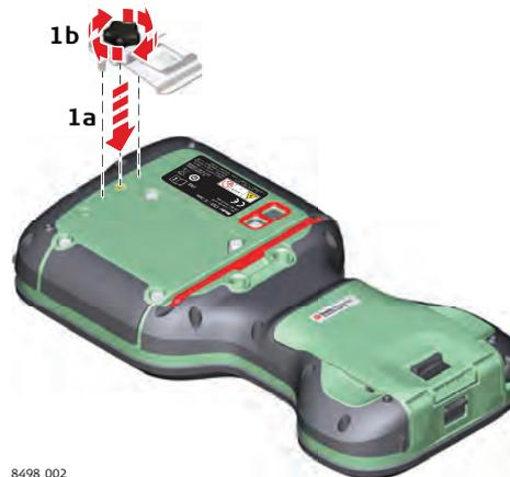
☞ If the hand strap is already attached to field controller, you need to detach it before you can fix the utility hook.
