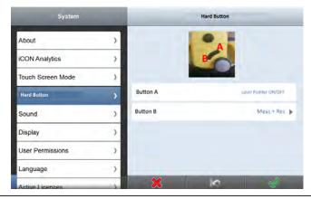
**Button A** is not configurable. This button turns the laser pointer on and off.
